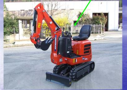
PROTECTION BAR ( it can be divided into two parts in order to enter in internal working sites ); On demand.
