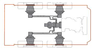
The gearboxes, compared with the traditional transmission by chain, which is subject to frequent repair and maintenance operations, have many advantages such as on elevated transfer speed (12 Km/h), homogenous distribution of the power directly on the wheels in favour of the force, a higher sensibility in the movements, the favourable possibility to work if need be, mounting old and new tyres on the same side without compromising the reliability of the machine.
