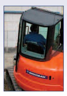
stick (and not on the pedal) in order to leave more room on the footboard, the seat is adjustable, the front glass has an opening mechanism given from gas springs, there is an efficient heating and ventilation system and, on request, the air conditioning system for a better thermic comfort during the whole year.
